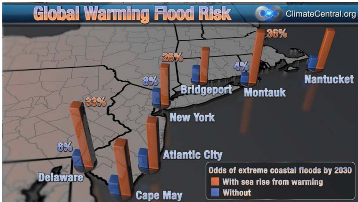
Figure 1. Odds of reference 100-year floods 2 when factoring in sea level rise from global warming, versus when not. See Table for source data.
